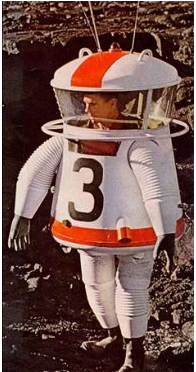
Space General Corporation's Lunar Exploration Suit, Model MK 1 during testing in the Mojave desert by the inventor Allyn B. Hazard. Here he is standing in a lava crater. The suit carried its own oxygen, food, and water. The suit stood eight feet high and weighed in at around 200 pounds
